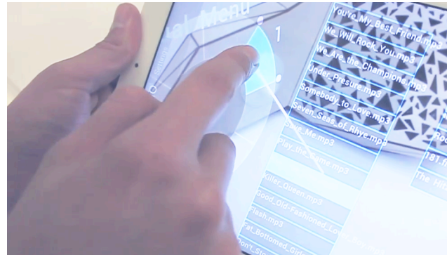
Figure 10: The chosen song gets dragged and dropped on a spot of the tuning knob. The action overrides the previously linked song or radio at this spot.
