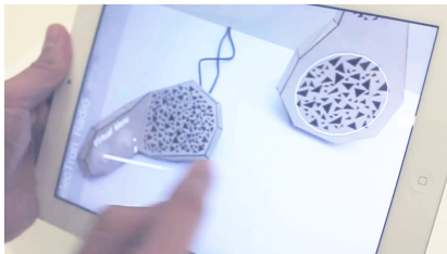
Figure 9: A user draws a line from the radio to a speaker in order to link the speaker with the radio.
