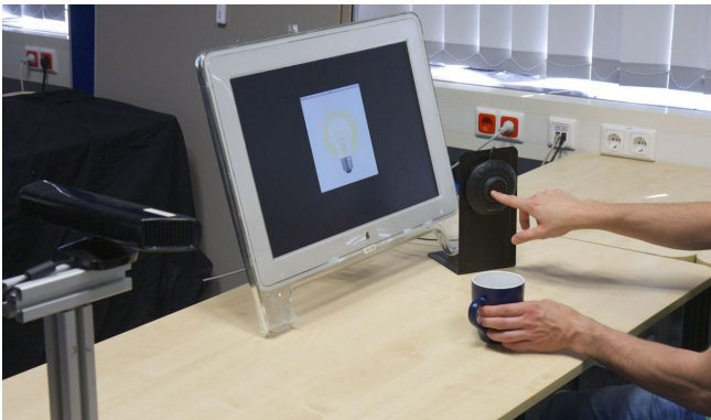
Figure 7. Setup of the system for the light scenario (left to right): Kinect, display, mug, rotary knob. The user is programming the mug by demonstration: mug and rotary knob used to control the light (on screen) are rotated at the same time. From now on, mug rotation dims the light.
