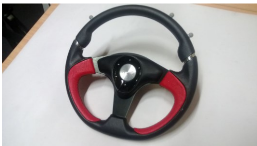
Figure 7: Passive steering wheel used as an active input device using tracking markers (visible on top)
