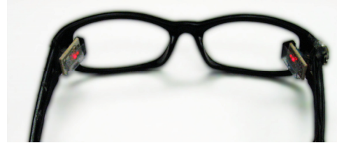
Figure 1. The wearable peripheral display.
