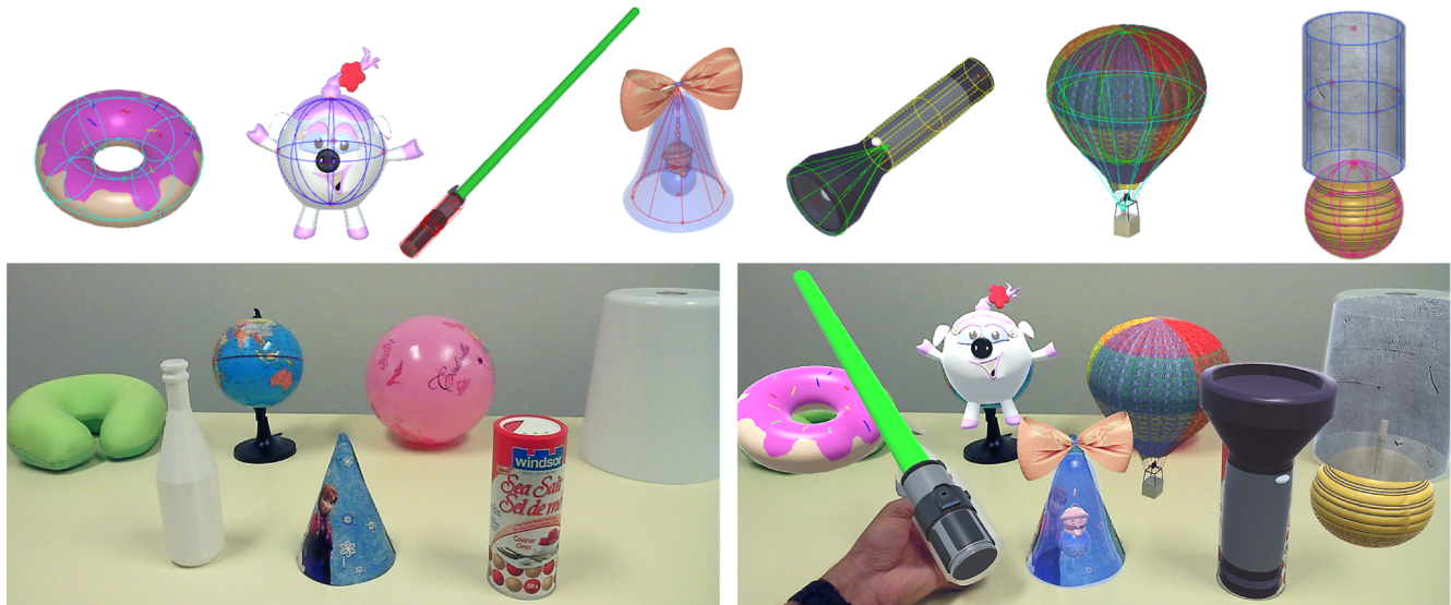
Figure 6: Top: the visual models used in our developer studies, overlaid with primitives from possible haptic models. Bottom: various visual models matched to physical objects based on the haptic models’ match for physical characteristics.
