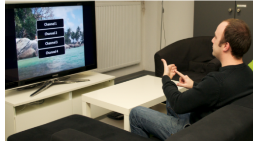
Figure 1. User taps on his non-dominant hand to operate the TV, while preserving his visual attention to the TV.
